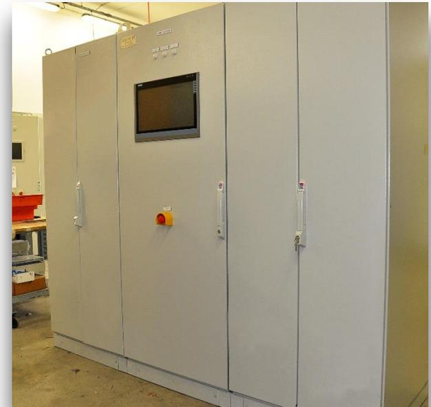
10 Unit Control Panel SIEMENS PLC based
