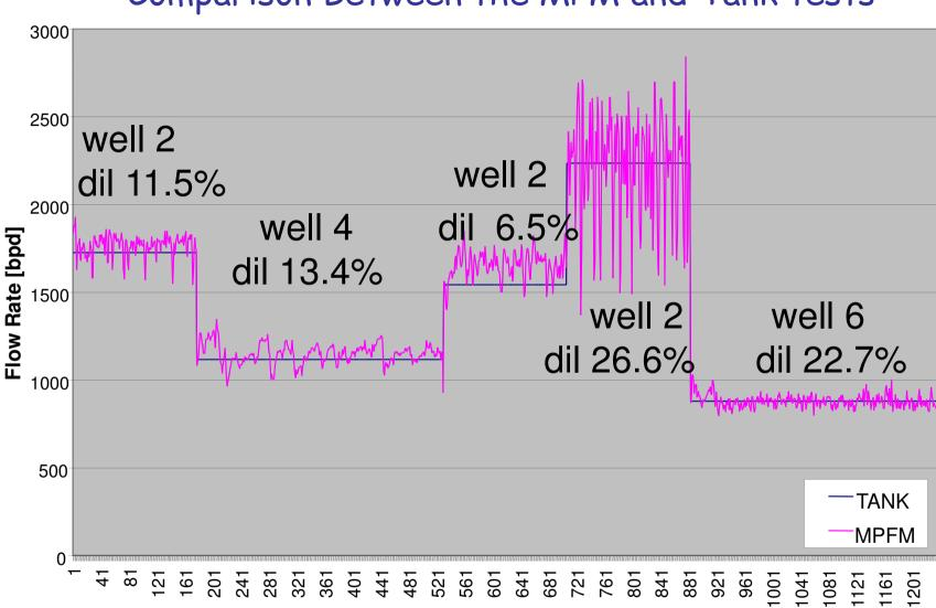
Comparison Between the MPM and Tank tests
