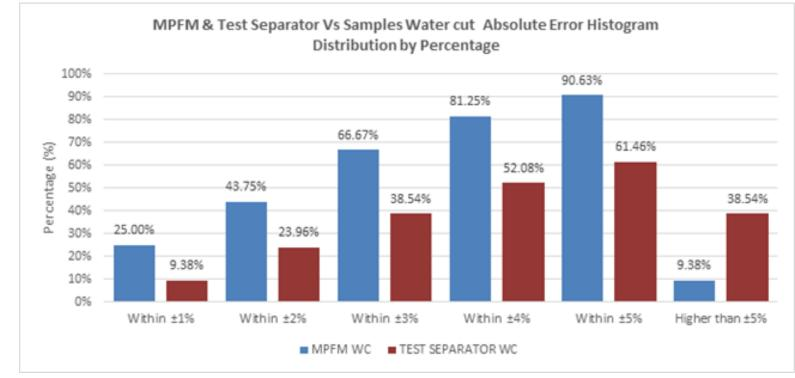
For the test separator, 61% of the data are within  $\pm 5\%$  (59 samples of total of 96)
