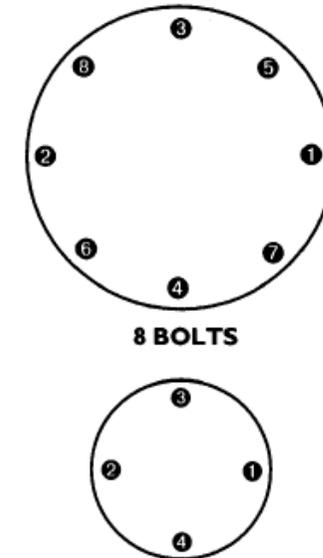
Figure 7: Bolt tightening sequence
