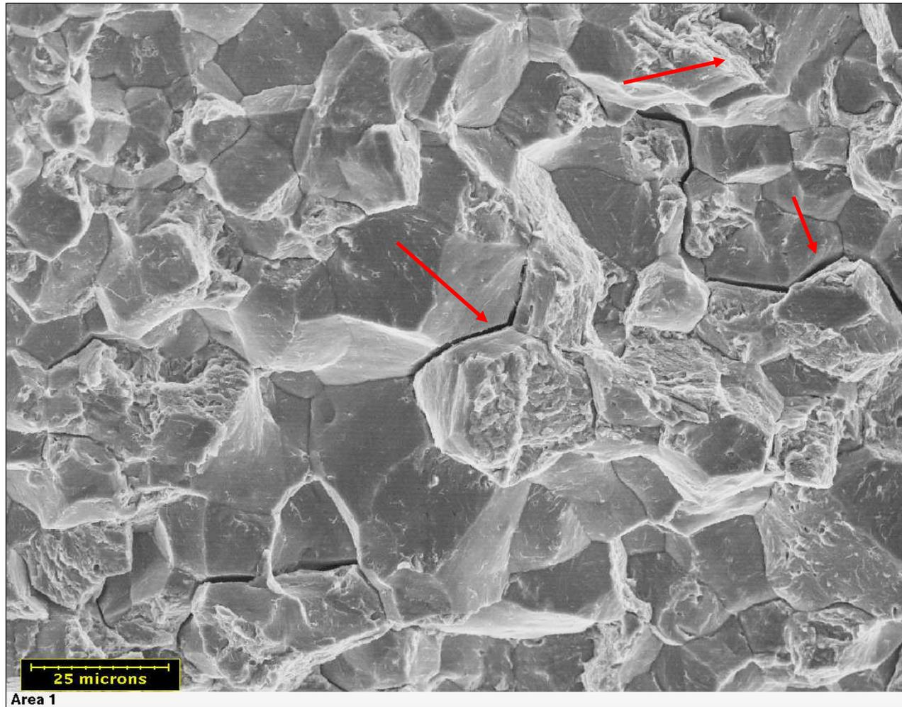
Hydrogen embrittled Carbon Steel (intergranular with secondary cracking)
