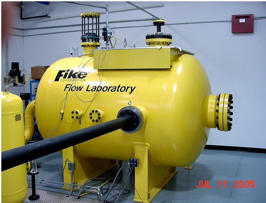
Large Zero-Velocity Vessel w/ 4" Flow Rig Attached
