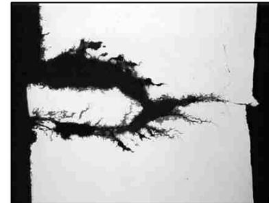
*Sulfide stress cracking*
