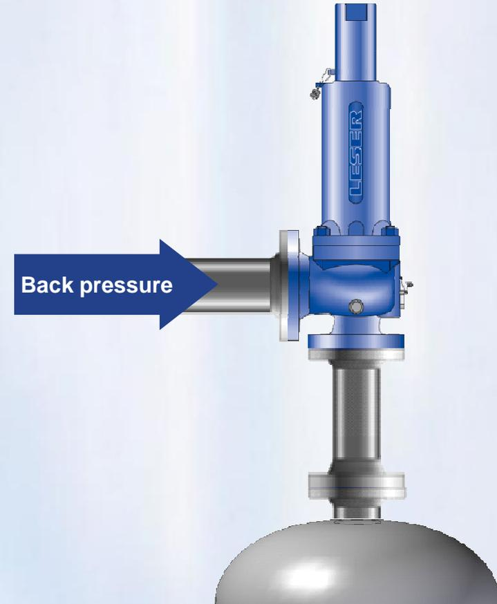
**Back pressure = built-up back pressure + superimposed back pressure**
