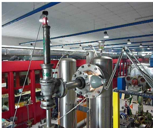
DN 1½" G 2½" during testing with water
