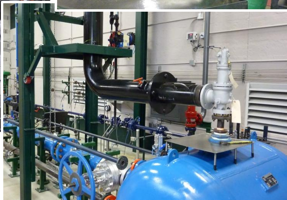
DN 2" J 3" during testing with nitrogen
