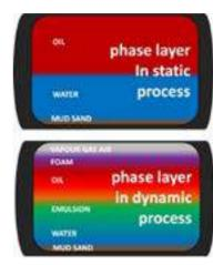
The reasons of all these considerations are in the density differences between each phase. By the way, also other parameters can influence the measurement (fluid composition and type of hydrocarbon present, salt concentration, turbidity, sand) while other could limit the compliance with some technologies (temperature, pressure, viscosity and velocity).
