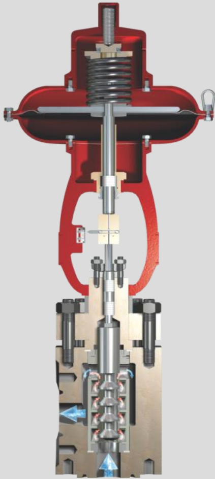
Typical multi-step design for liquid service, with relatively larger flow area compared to stack technology valves.
