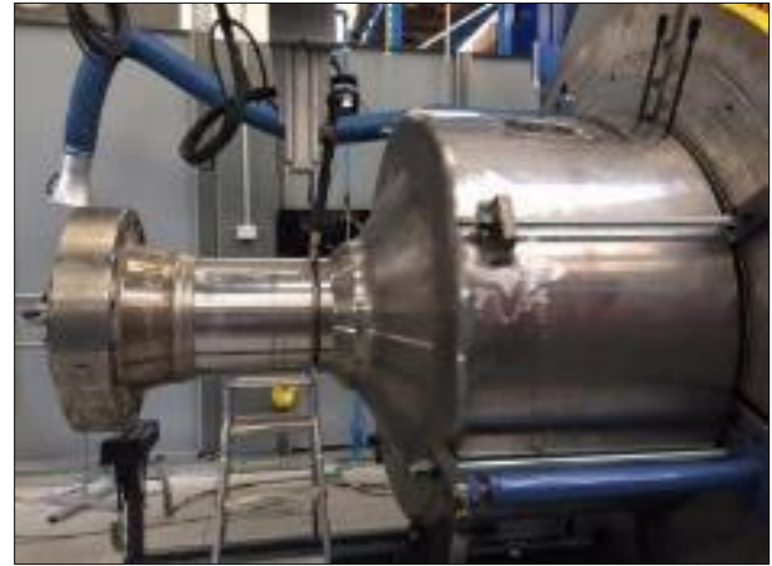
(GTAW) WELDING PUP IN SDUPLEX TO VALVE BODY IN F60 W/ALLOY 59
