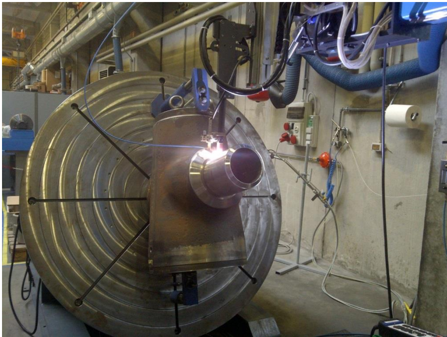
(GTAW) WELDING PUP IN SDUPLEX TO VALVE BODY IN F60 W/ALLOY 59
