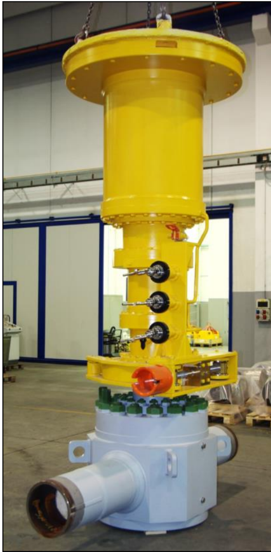
SSIV 14" Class API 1500 c/w ROV retrievable actuator
