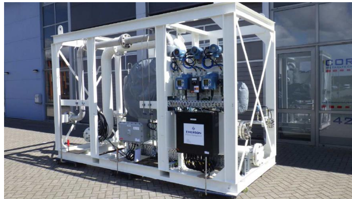
The skid allows for mass flow based Emerson Coriolis MID flow meter assessment.
